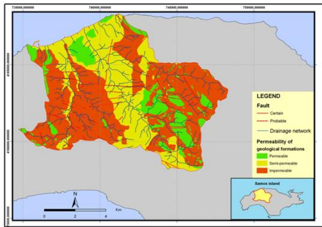
**Figure 3:** Permeability of geological formations of the Karlovassi graben.
